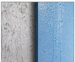
Compared to common plastic surfaces, Craemer **Palgrip**<sup>®</sup> anti-slip sheets offer absolute slip resistance even in high humidity thanks to their high quality grain structure.
